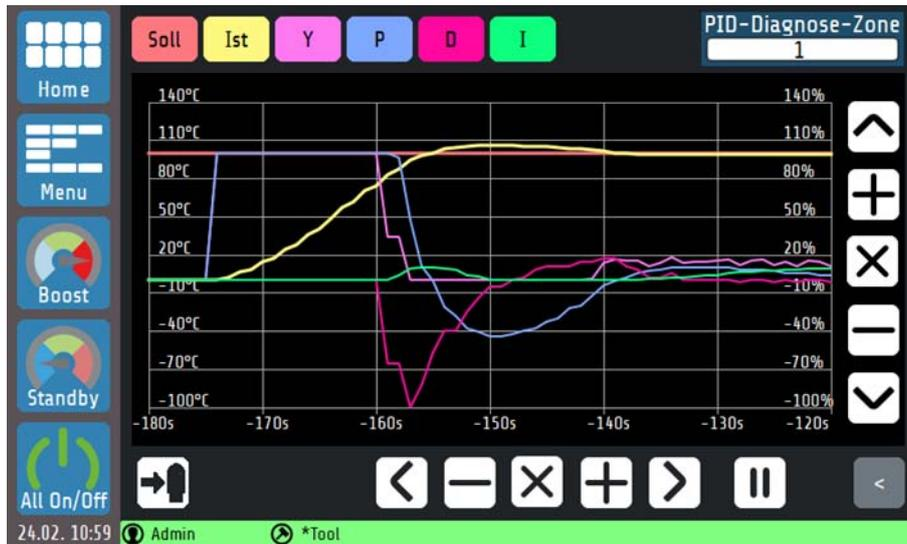
This view shows the temperature curve and the gradients of the P, I and D components for a selected zone. In this way, the influences of the three control parameters on the process can be explored and conclusions can be drawn about the output ratio generation. The control elements for scaling the graph behave as shown in chapter 10. Explanation of the individual boxes:
