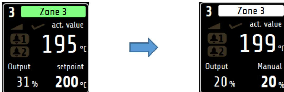
The zone now no longer follows colour coding, but is permanently displayed in white. The set manual output ratio is displayed instead of the setpoint. The manual output ratio can be entered in the Home screen (Home) by tapping the zone tile.
