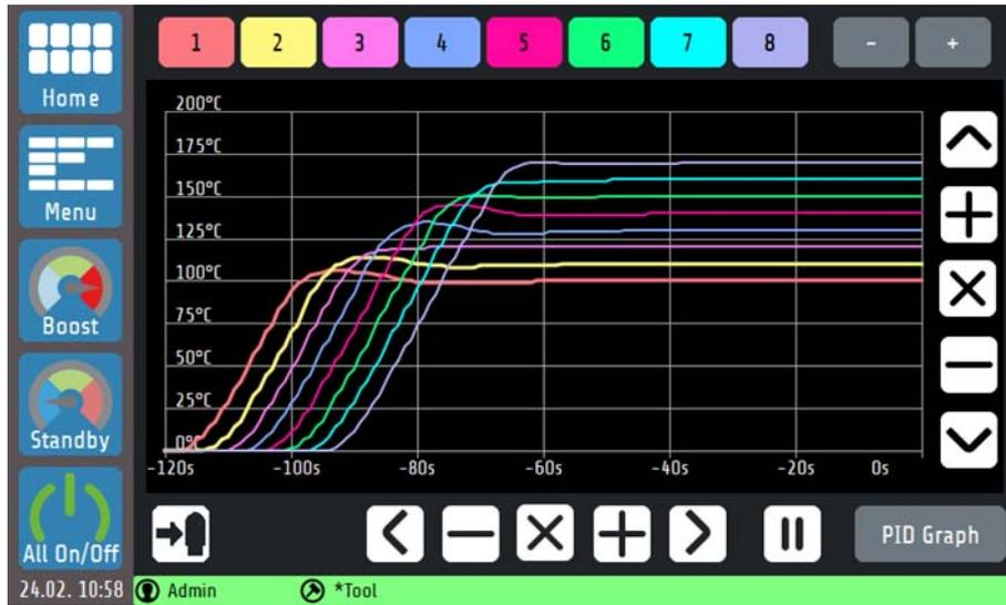
The curves of all zones can be saved immediately to a USB flash drive via the USB export button. Explanations for the individual boxes:
