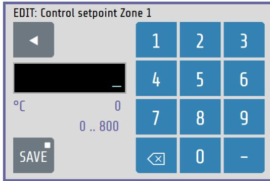
The parameter name of the zone (here: **Control Setpoint Zone 1**) is displayed in the header.
