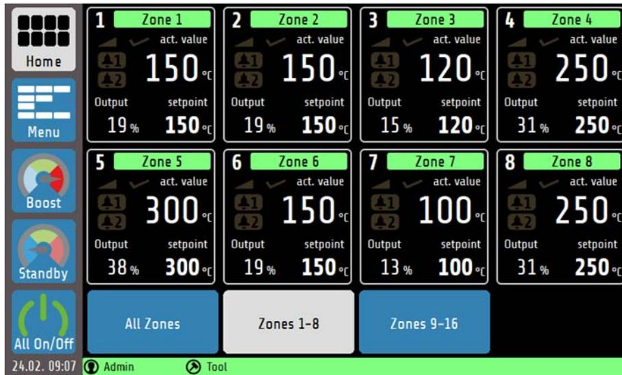
The home screen can be switched between the view of zones 1-8, 9-16 and a view of all available zones. The 8-zone view has the highest information content, while the **All Zones** screen only shows the target and actual values as well as the signal display. Explanation of the individual boxes:
