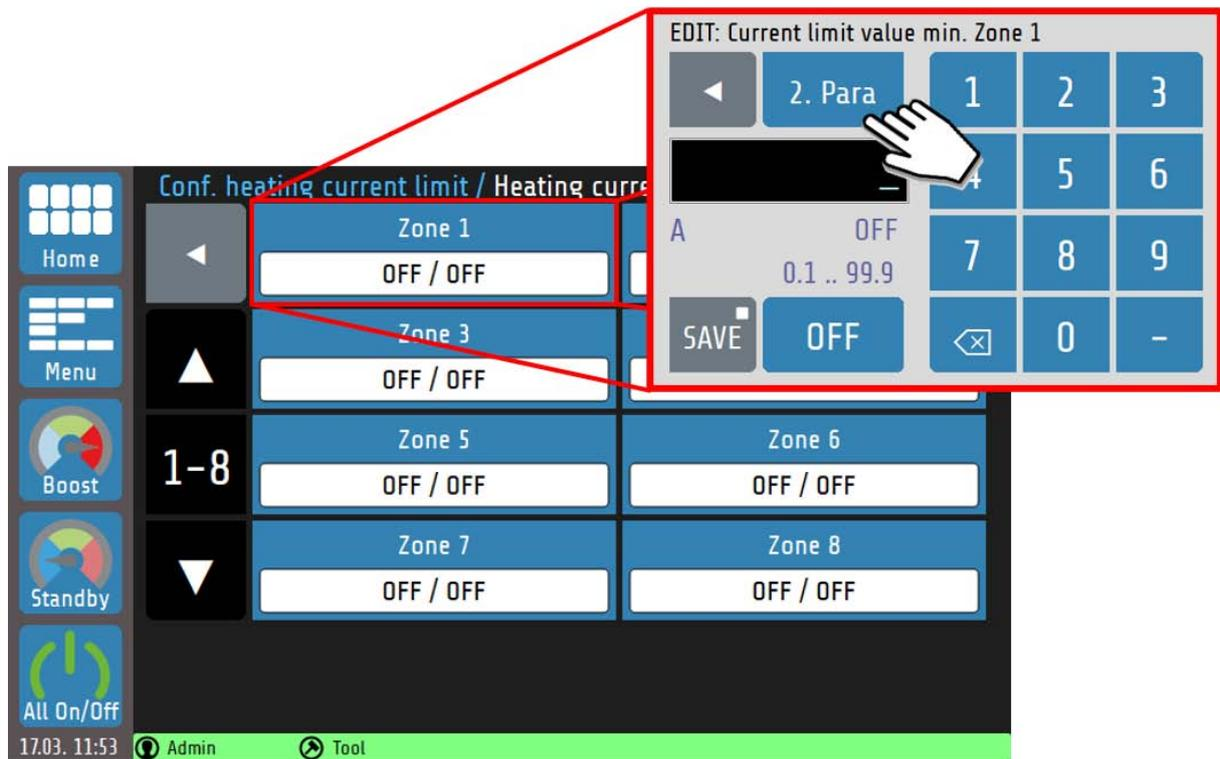
The **minimum current limit value** is set first during the limit value configuration. Application: Detection of the failure of a heater. For systems with several heaters per zone, a partial failure can be detected.
