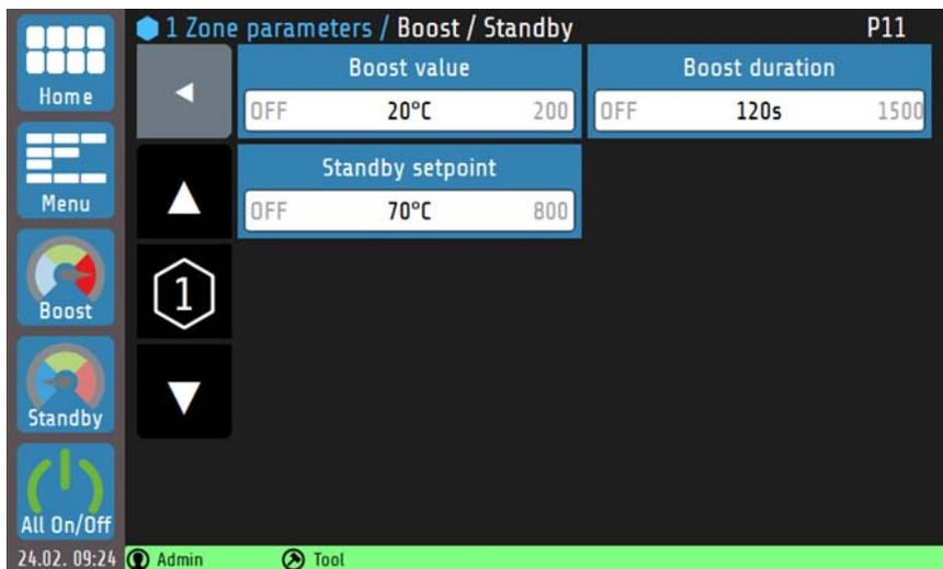
The **Boost** and **Standby** function can be started or stopped from the **navigation bar**. The zones whose **boost** and/or **standby** parameters are set to **OFF** are not affected when enabling the global boost/standby. For more information on the **Standby** and **Boost** function, see Chapter [15.4](#).
