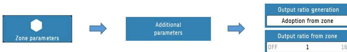
The parallel connection allows the work process to be continued with a correct function and terminated to subsequently carry out repair. The coupling of zones causes the defective zone to take over the **output ratio** of an intact zone.
