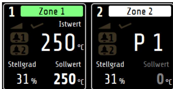
A coupled zone is symbolised on the **home screen** by a white bar within the **zone tile**. Instead of the actual value, this zone contains a **P** (for **parallel connection**) and the number of the coupled zone (here: **Zone 1**)
