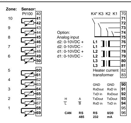
It is not permitted to connect the grounds of the sensor-inputs and bist. voltage-outputs with each other.
