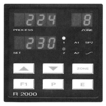
**LED 1:** Control output "heating" of the choosen zone active LED 2:
