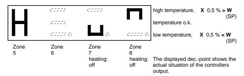
Zone 5: H = Manual output ratio. Flashing: sensor error (see page 14)
