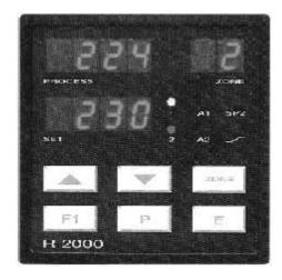
LED A1: Alarm 1 activ LED SP2: Setpoint 2 valid LED\_\_\_\_: Ramp function activ LED 1: Control output "heating" active LED 2: Control output "cooling" active LED A2: Alarm 2 activ
