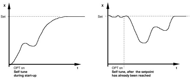
Self-tuning can be stopped by selecting the option OPT = OFF and pressing the "E" - key.
