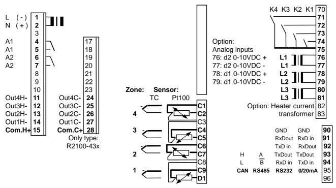
It is not permitted to connect the grounds of the sensor-inputs and bist. voltage-outputs with each other.
