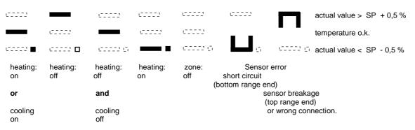
The flashing dec.-point shows, that either "heating"- or "cooling"-output is active.
