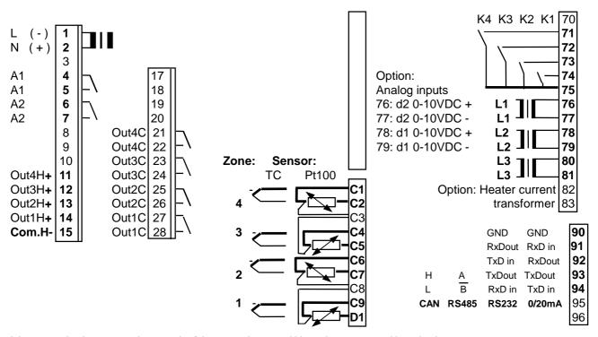
It is not permitted to connect the grounds of the sensor-inputs and bist. voltage-outputs with each other.
