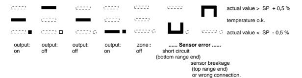
The flashing dec.-point shows, that the control output is active.
