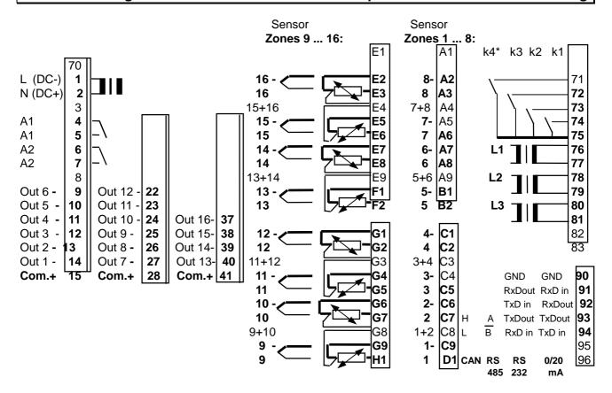
It is not permitted to connect the grounds of the sensor-inputs and bist. voltage-outputs with each other.
