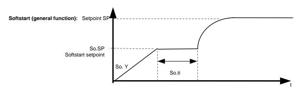
During the softstart the controllers' output response is limited to a pre-selected ratio, in order to achieve a slow baking out of high performance heat cartridges.
