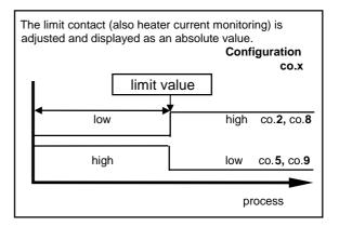
The alarm relay of the limit comparator with start-up suppression is activated when the controller is first switched on. It is only then deactivated, when the process value has been within, and left, the o.k. -zone. Configuration co.x limit range high. low high co. 7 setpoint process
