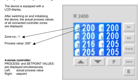
Most of the individual parameters of the device are displayed in plain text either in english or in german. See chapter 6: Device Configuration (press keys "E" and "P" simultaneously for appr. 3 seconds).
