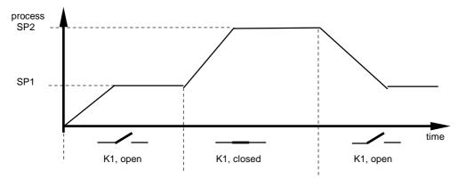
Alarm A1: Alarm value (switches relay A1) Temperature monitoring:
